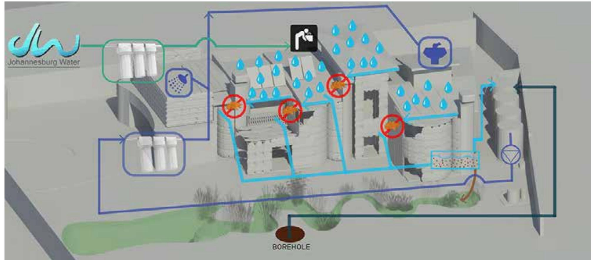
IMAGE 12: RAINWATER COLLECTION SYSTEM
